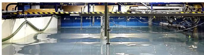
Siya Jin [1] - Physical scenario in the laboratory. The cylindrical buoy installed in the centred area is the experimental 1/50 scale PAWEC device
