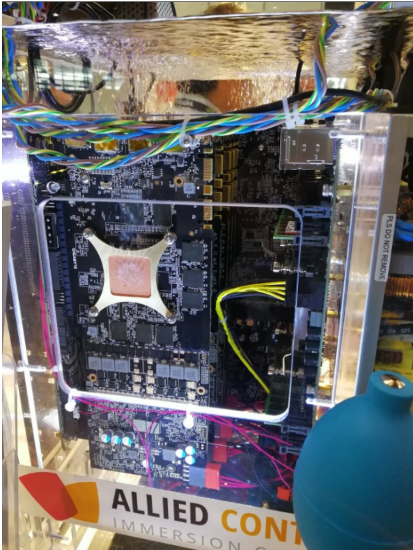
An example of immersion cooling, an alternative to air cooling in the data centre
